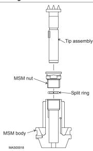
Figure 91: Reassemble MSM Nozzle
