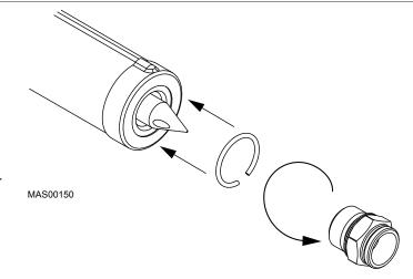
Step 7: Place snap ring over the tip and screw down the nut. The snap ring should "snap" into place around the nut. See the X Range Nozzles Torque Setting table for the correct torque for the nut.
