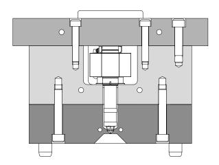
Figure 12: Suggested Placement of Clamping Bolts
