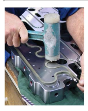
Figure 50: Hammering in a Pressed-in Heater
