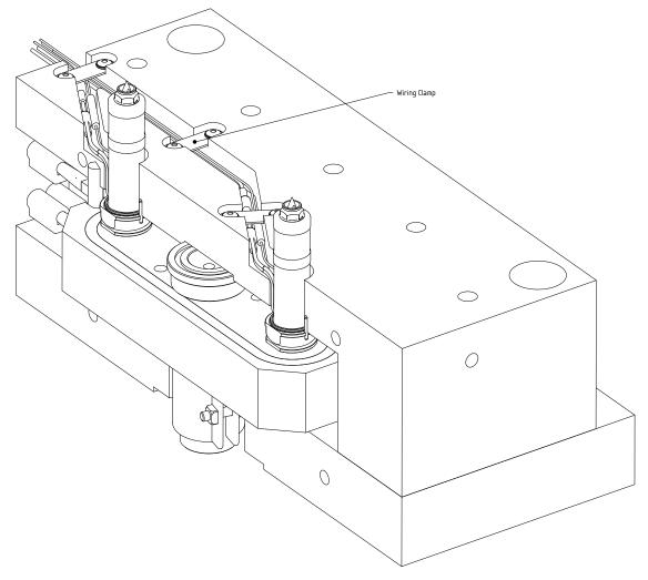
Figure 17: Manifold Wiring Diagram (Cutaway view)
