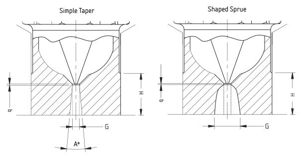
Figure 4: Sprue Nut Gate Land Modification Examples
