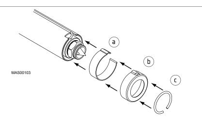
Figure 81: Replace BX or SX T/C Clip, Heater Cap, and Snap Ring
