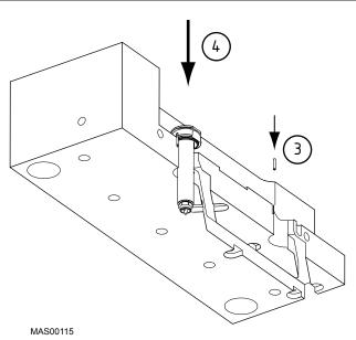
Figure 29: Insert Dowels and MX Nozzles
