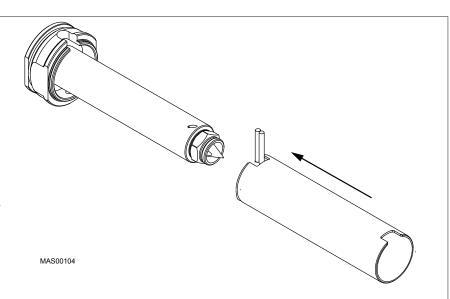
Figure 72: Slide Heater on MX Nozzle
