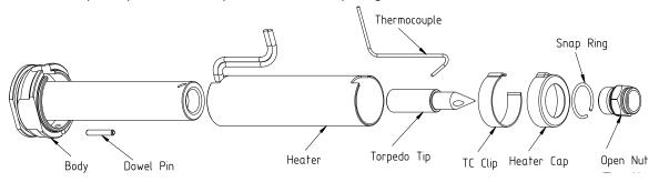
Figure 55: Parts of a MX Nozzle
