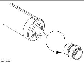
Figure 60: Unscrew Nut on an X Range Nozzle
