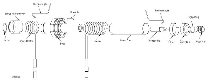
Figure 56: Parts of an SX Nozzle
