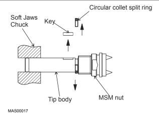
Figure 90: Remove MSM Key and Collet Halves
