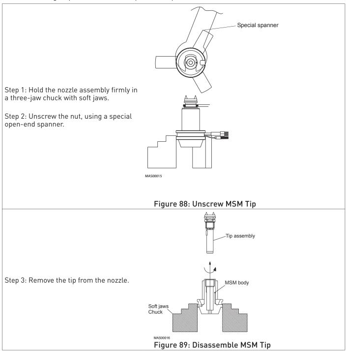
Step 4: Firmly hold the tip assembly with a three jaw chuck with soft jaws.
