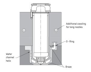
Figure 15: Insert with Helical Cooling Channels Example
