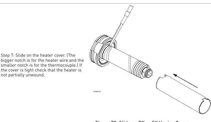
Figure 79: Slide on BX or SX Heater Cover
