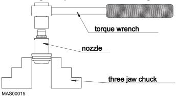
Figure 87: Correct Placement of a Nozzle in a Three Jaw Chuck
