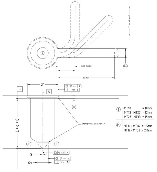
Figure 19: MT Range Nozzle Installation Tolerances
