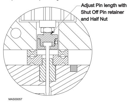
Figure 43: Valve Cylinder Front Face
