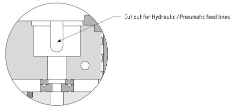
Figure 2: Slots for Feed Lines
