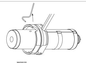
Figure 84: Replace SX Sprue Thermocouple
