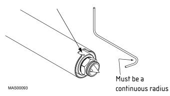
Figure 73: Install Thermocouple on MX Nozzle
