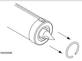
Figure 61: Remove Snap Ring on an X Range Nozzle
