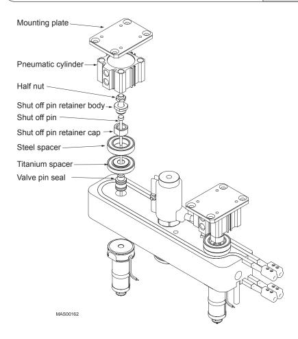
Figure 42: Complete Valve Gate Assembly
