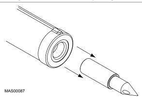
Figure 62: Remove Tip on an X Range Nozzle
