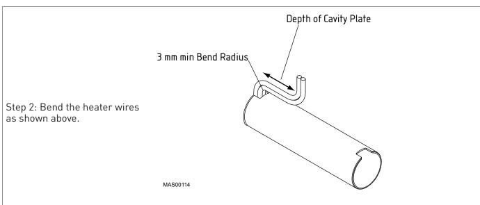
Figure 28: Bend MX Heater Wires
