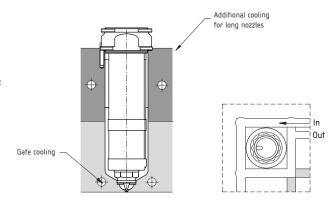
Figure 13: Cooling Channels Example
