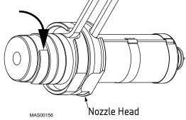
Figure 83: Remove SX Sprue Heater
