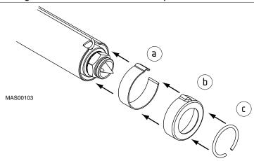
Figure 74: Re-install T/C Clip, Heater Cap, and Snap Ring on an MX Nozzle
