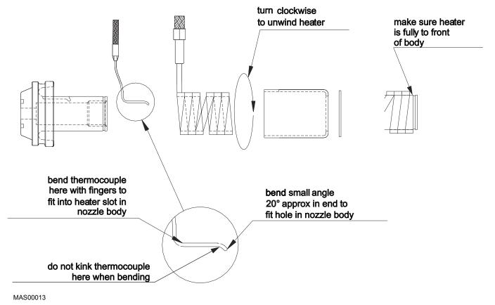
Figure 86: MT Nozzle Thermocouple and Heater Replacement
