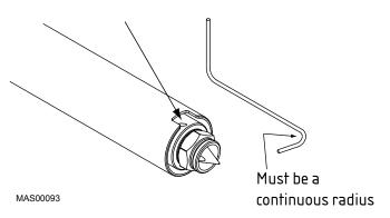
Figure 67: Install Thermocouple on an X Range Nozzle
