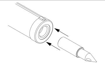
Step 6: Ensure hole in body is clear of any plastic or obstructions and gently slide the tip into the assembly.
