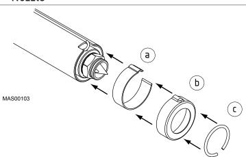
Figure 68: Install T/C Clip, Heater Cap, and Snap Ring on an X Range Nozzle
