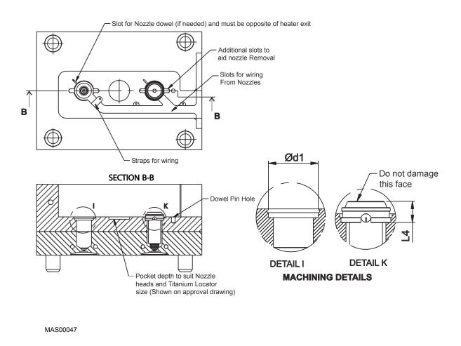
Figure 39: Detail of the MT Nozzle Range in Manifold
