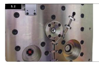
Fit the back plate cap screws and torqe screws evenly from the centre out. Fit the wire clips to the wire grooves and ensure the wiring is tidy and free from any areas that may pinch or damage the cables. Fit the locating ring.
