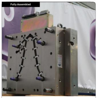
Fully assembled hot half showing nozzles, wire slots and wire clamps
