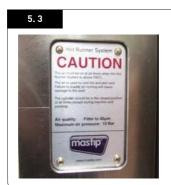
Fit the name plates and caution plates using the hammer drive rivets.
