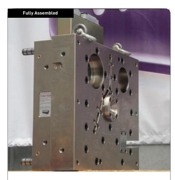
Fully assembled hot half from sprue side.
