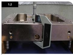
Measure plate thickness Measure the overall thickness of the manifold housing plate with a micrometer. → Record measurements
