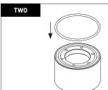
Fit the Cylinder End Seal 13 to the Cylinder 12 Apply grease\* to Cylinder End Seal 13
