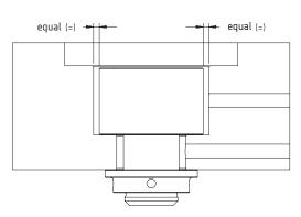
Centralise **Cylinder Assembly**  $\boxed{A}$  to the Actuator pocket.
