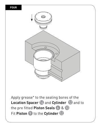
$<sup>^{</sup>st}$  Mastip recommends using high temperature silicon grease
