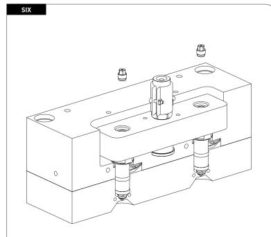
Clean any residue material from the pin seal pocket and thread in the manifold.
