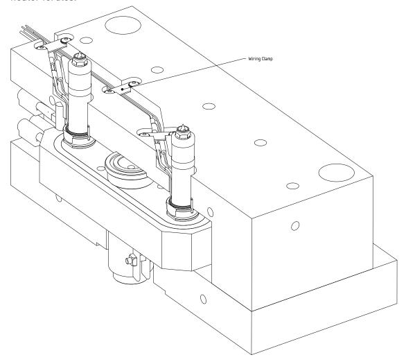
Figure 17: Manifold Wiring Diagram (Cutaway view)
