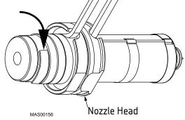
Figure 83: Remove SX Sprue Heater
