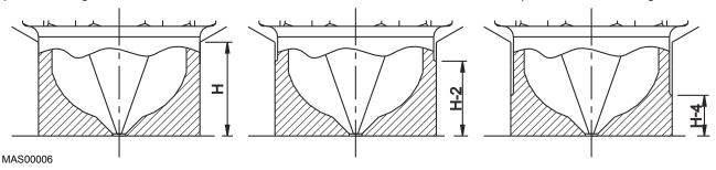
Figure 92: Example of Heat Build Up in Sprue or Bush Nuts
