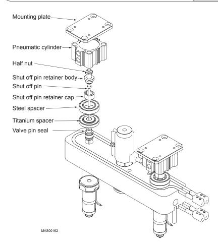
Figure 42: Complete Valve Gate Assembly
