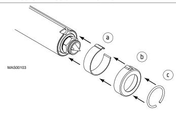
Step 3: Install the T/C clip (a), the heater cap (b), and the snap ring (c) (in that order).
