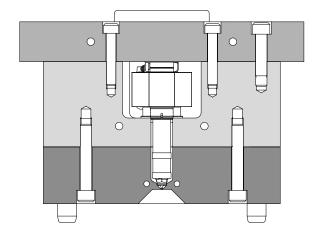
Figure 12: Suggested Placement of Clamping Bolts
