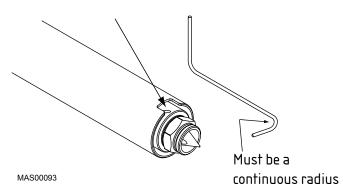
Figure 73: Install Thermocouple on MX Nozzle
