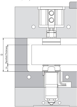
Figure 7: Measurements Needed for Manifold Expansion Calculation (Valve Gate)
