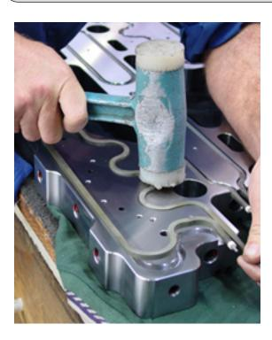
Figure 50: Hammering in a Pressed-in Heater
