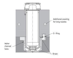
Figure 15: Insert with Helical Cooling Channels Example
