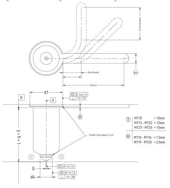
Figure 19: MT Range Nozzle Installation Tolerances
