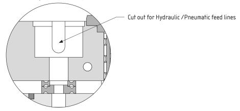
Figure 2: Slots for Feed Lines
