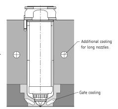
Figure 14: Insert with Cooling Channel Groove Example
