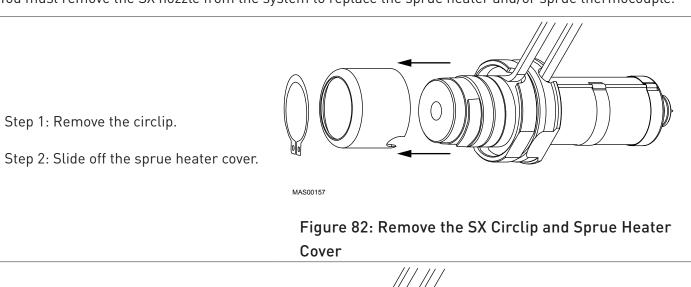
Step 3: Grip the nozzle head and remove the coil heater by turning the tip end of the heater in a clockwise direction to "unwind" or loosen the heater coils, and at the same time pull the heater off the body.
