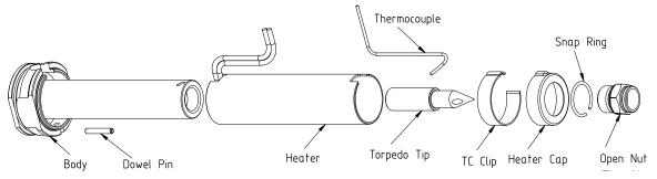
Figure 55: Parts of a MX Nozzle
