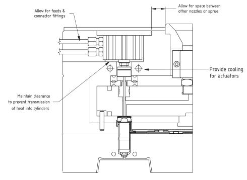
Figure 11: Mould Modifications for Valve Gate Applications
