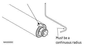
Figure 80: Replace BX or SX Thermocouple
