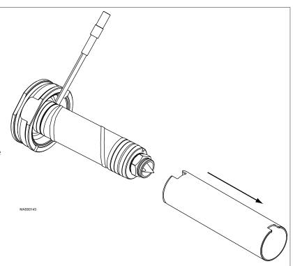
Step 3: Slide off the heater cover (leave the tip and the nut in the nozzle).
