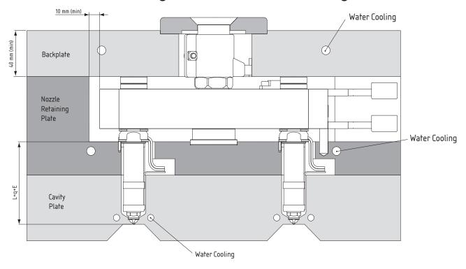
Figure 1: Example Layout for a High Production Manifold
