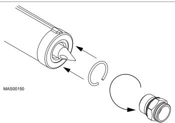
Figure 64: Replace Snap Ring and Nut on an X Range Nozzle
