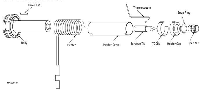
Figure 54: Parts of a BX Nozzle
