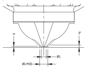
Figure 3: Increasing the Open Nut Gate Land
