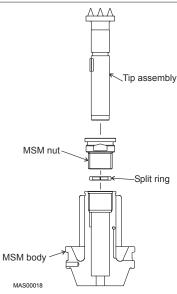
Figure 91: Reassemble MSM Nozzle
