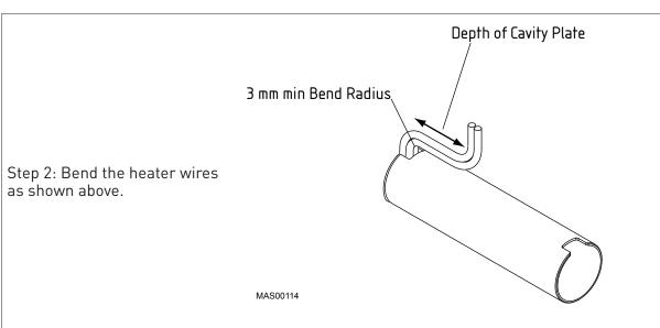
Figure 28: Bend MX Heater Wires
