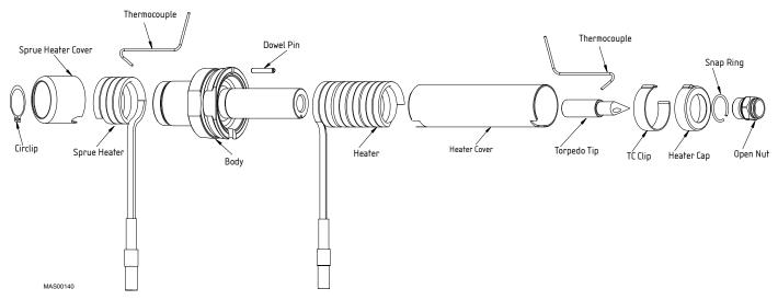
Figure 56: Parts of an SX Nozzle
