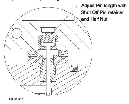
Figure 43: Valve Cylinder Front Face
