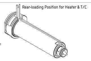
Step 2: Bend the T/C along the outside of heater and bend it again with the heater wires at the nozzle head.
