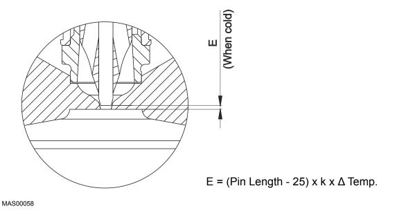
Figure 44: Gap between Gate and Pin
