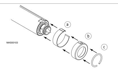
Figure 81: Replace BX or SX T/C Clip, Heater Cap, and Snap Ring
