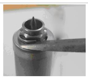
Figure 57: Wedge a blade under a X Range Nozzle Snap Ring
