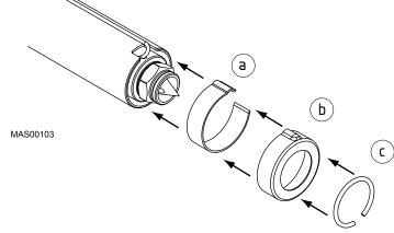
Figure 74: Re-install T/C Clip, Heater Cap, and Snap Ring on an MX Nozzle
