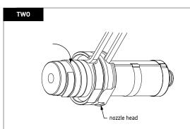
REMOVE OLD **SPURE HEATER** - Grip the **nozzle head** and turn the **heater** in a clockwise direction to unwind or loosen the **heater coils**. Simultaneously pull the heater off the body
