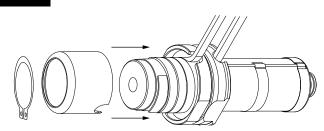
Install New Heater - With bottom **heater** connection in line with slot on body, push the **heater cover** as far as it will go onto the **nozzle body**. Turn the tip end of the **heater** in a clockwise direction to unwind or loosen the **heater coils**. Simultaneously push the **heater** towards the head of the **nozzle**. Make sure the **heater** is fully forward on body.
