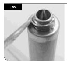
Twist the end of the tool towards the end of the nut so that the end of the snap ring rides up out of the groove and over the nut shoulder.
