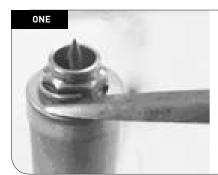
Locate the ends of the snap ring.
