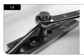
Place a spanner around the nut and place a soft pry bar under the hex of the hut. Simultaneously lever upwards with the soft pry bar and turn the nut with the spanner. Patiently work the nut upward while the plastic is molten. If the plastic cools and prevents the nut coming off, apply more heat to the nut to return plastic to molten state.
