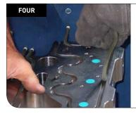
To remove straight heater sections pull on heater ends and bend it out of heater slot.
