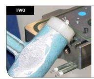
Using a hammer and a plastic wedge between the heater and the bottom of the slot, pry the heater out of the slot. Work from the ends of the heater towards the centre.
