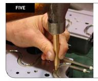
Gently tapping with a soft aluminium tool and hammer slightly indents the heater face, giving it a tight fit in the heater slot.
