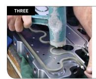
Starting at the centre of the heater and working towards the heater ends, use a soft-faced hammer to lightly tap the heater into the slot until the heater is sitting just below the manifold.
