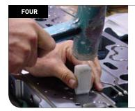
Using a hammer and a soft aluminium or brass tool (see below) gently tap the heater top until it is approximately 1 mm below the manifold face. Repeat this action working along towards the heater ends until the heater has been pressed in
